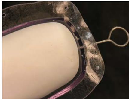
Place the second half of the mold on the model and bolt the halves together.
