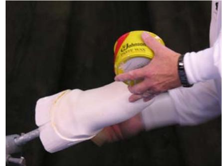
Place the mold half with the alignment pin first. This will make it easier to find the corresponding hole in the cast without damaging the cast with a miss
