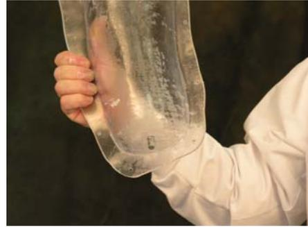
Wax or Vaseline can be worked into the cast to fill the smallest of defects. Any marks left will be faithfully reproduced in the finished liner
