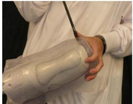
If the plastic is at the right temperature and the vacuum strong enough during forming, the seam as viewed from the inside, will be minimized
