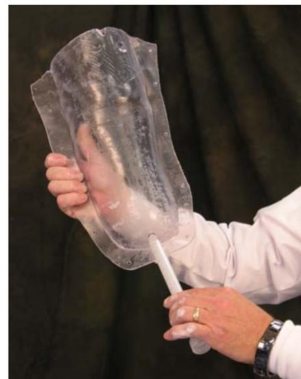
Fit the injection hole with a threaded tapered plug
