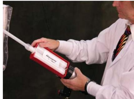
The silicone can be dispensed by hand or pneumatically using injection guns designed to accept the side by side
