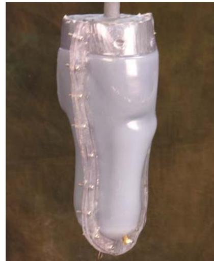
Check the cure time of the silicone being used before opening the mold. All the platinum cure silicones can have their cure time accelerated by the application of heat if necessary. A large heating pad works well.
