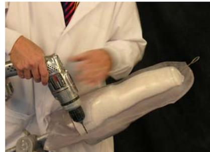
Drill a series of holes through both sides of the newly formed mold. These holes will be used later to bolt the mold back together. Try and drill the holes as close to the model as possible. This will help prevent the silicone from being forced between the two mold halves
