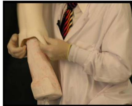
Inspect the inner casting for any defect. The smallest bubble in the casting will result in a corresponding bump on the inside of the finished product. The liquid silicone has an unbelievable ability to fill even the smallest cavity.
