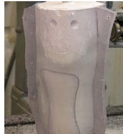
The two halves can now be separated. The protective covering that was left in now serves as the parting agent. It will be necessary to separate the two halves with a screwdriver the first time.
