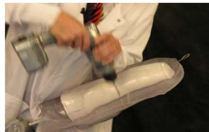
This photo shows the distal pin in place , all bolt holes and the final trim before the halves are separated
