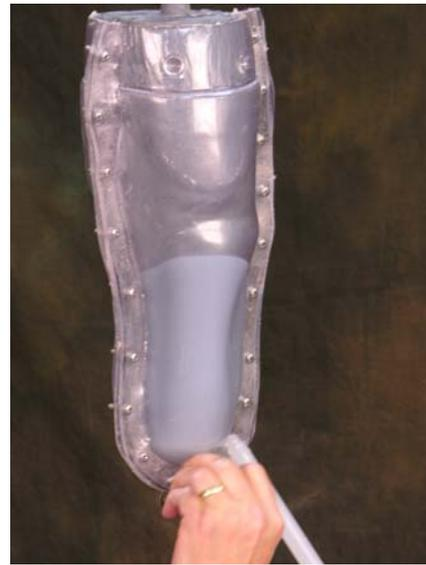
The mold is now completely filled. The silicone should completely fill the vents created at an earlier step. This extra bit of silicone becomes necessary if there is any leakage when the static mixing nozzle is removed and the threaded plug inserted.
