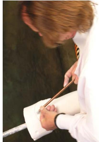
Pick a low point on the outer mold half as a starting point for the injection of the silicone. Make the hole just large enough to accept the static mixing nozzle without allowing it to enter too far into the mold
