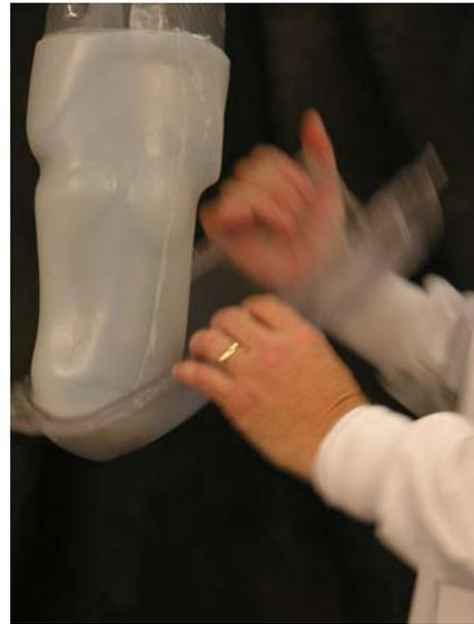
The finished liner will probably require trimming any silicone that was forced between the mold halves. (flashing)
