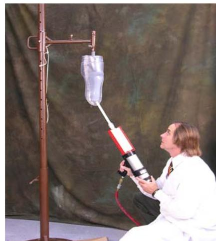
The cast has been painted gray for contrast so you can see how the mold is filled from the bottom to the top. This helps to reduce the chance of any bubbles being trapped during the injection process
