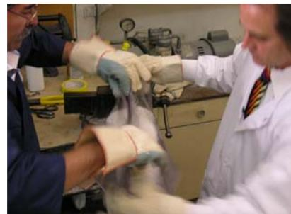
Try and follow the target seam line as close as possible. Keep the two pieces of plastic as smooth and flat as possible as the plastic cools
