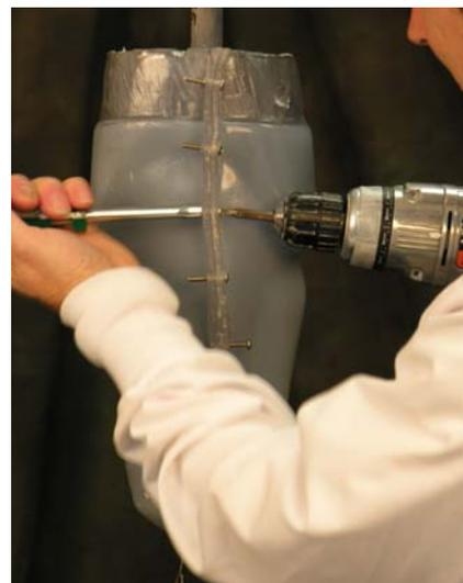
As soon as the silicone has cured it is safe to remove the mold halves. Do not forget to remove the distal alignment pin.
