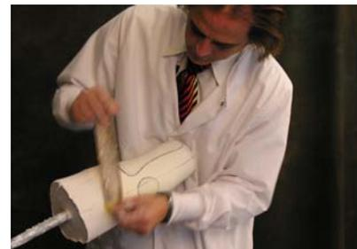
Make registration dimples in the cast with a large drill bit. This helps to align the outer mold halves to the inner model. Place two depressions on the anterior and two on the posterior sides of the model.
