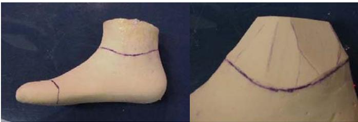
After drawing trim lines as desired. Angle the top of the cast. Start at the trim line and angle toward the bolt hole. These angles are used to prevent rotation of the plug when bolted to the top of the mold.
