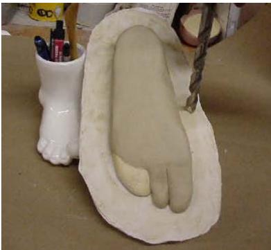
When the top of the mold is done, completely remove the water based clay from the plaster top portion. Use a large  $\frac{3}{8}$ " –  $\frac{1}{2}$ " (10-12mm) drill bit to create "dimples" in the plaster to register the top and bottom of the mold.
