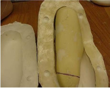
Clean the clay from the plaster mold insert and outer mold parts. Bolt the in the insert and reassemble mold parts. Drill a ½” hole in the top of the mold at the heel area for the injection nozzle, and small holes at the end of each toe to allow air to escape. The silicone you are going to inject must have a way to escape when the mold is full. Allow the silicone to fully cure (approx. 4 hours) before demolding.
