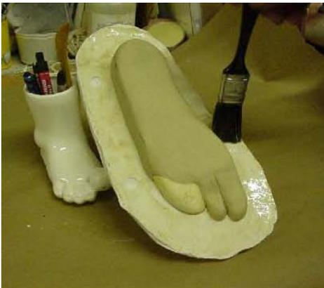
Apply parting agent on any area where plaster might stick. Make a "dam" around the top portion or the mold to form a mold for the bottom portion. Fill the bottom of the mold with plaster of paris, and allow the plaster to dry.
