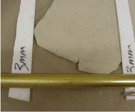
3mm clay is being used for the top of the foot. This is the suggested thickness, but you can use any thickness to reach the desired effect.
