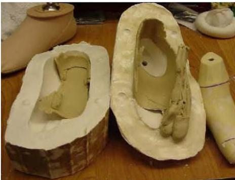
Top and bottom of separated mold.
