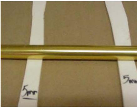
Roll clay to the desired thickness. (5mm works well). The photograph shows 5mm Pelite being used as a guide. Turn the clay often so it does not stick to the paper. Make the 5mm slab larger than the insole pattern.
