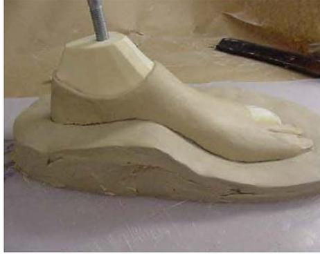
Apply parting agent on any area where the plaster of paris might stick. Apply plaster to form the upper part of the mold. The first layer of plaster of paris should be applied with a brush to eliminate bubbles and completely cover the details in the toe sculpture.
