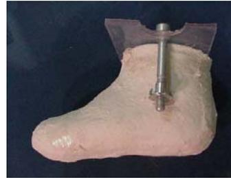
Make a plastic holder for an  $\frac{3}{8}$ " ankle bolt and T-Nut assembly, thread the T-Nut up  $\frac{1}{2}$ " (12mm) which will hold the insert in place during fabrication steps.
