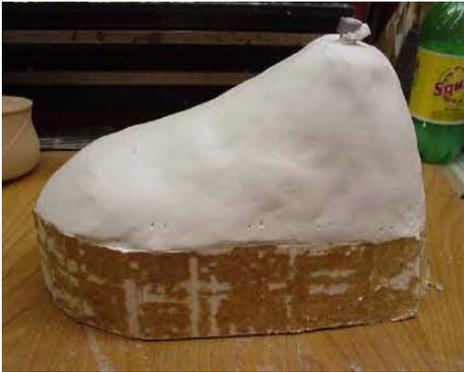
Completed mold looks like this. Remove the bolt and open the mold by working along the seam with a screwdriver or other flat tool.
